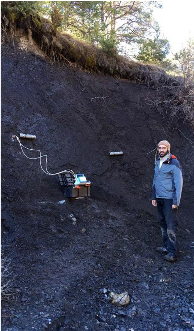
**Figure 1A.** EGM-5 Portable CO<sub>2</sub> Gas Analyzer connected to a chamber drilled in the rock face [2], through the MS<sup>3</sup> monitoring-sampling system [3], while we measure CO<sub>2</sub> efflux from sedimentary rock in the Laval stream catchment, Draix, France. (© R. Hilton)
