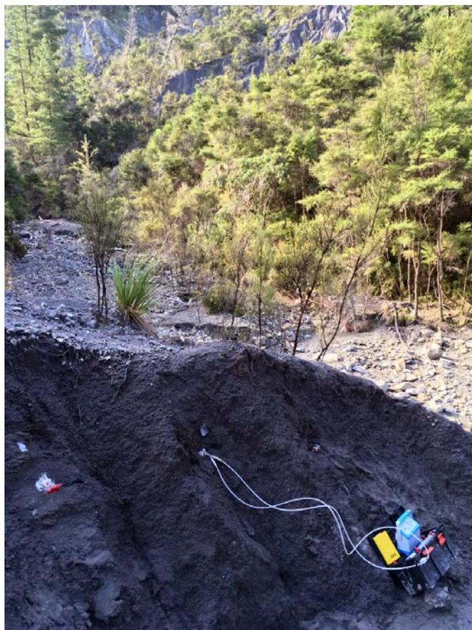
**Figure 2.** An example of the new method (EGM-5 Portable CO<sub>2</sub> Gas Analyzer connected to a chamber drilled in the rock face [2], through the MS<sup>3</sup> monitoring-sampling system [3]) being used in the Waiapu River catchment, New Zealand. (© R. Hilton)
